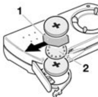
As a protection against discharge two 3 volt battery cells are separated by insulating paper (1). Remove paper on commissioning. Take care that the contact sheet (2) remains between the batteries.
