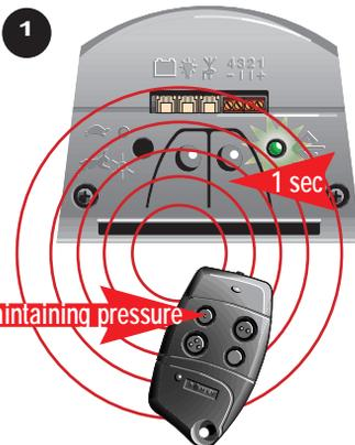
**1** Press and hold the remote control button the press the adjustment push-button briefly to memorise the remote control buttons.
