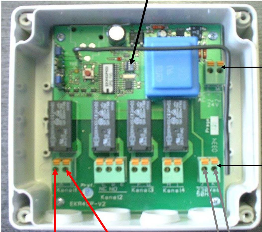
Optional 24v Power Connection (use as an alternative to the 240 V connections below)
